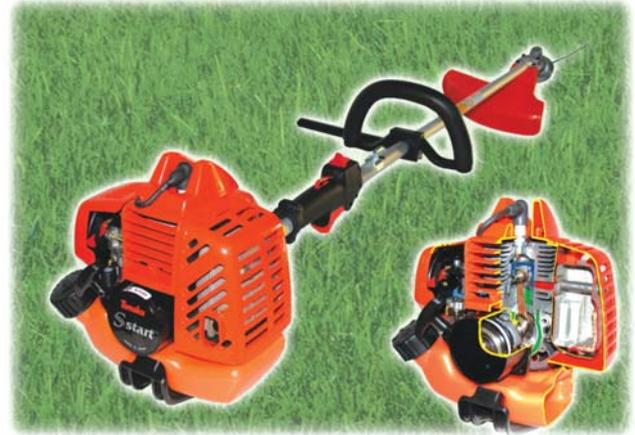
The Tanaka TBC270S brushcutter sports a PureFire engine (inset) that's 30% more fuel efficient and which reduces emissions by up to 70%.
