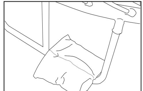
Figure 22-C: Placing the sandbag over the leg
