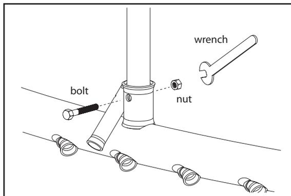
Figure 5: Fastening the legs to the frame
