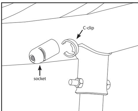
Figure 21: C-clip attaching to socket on frame
