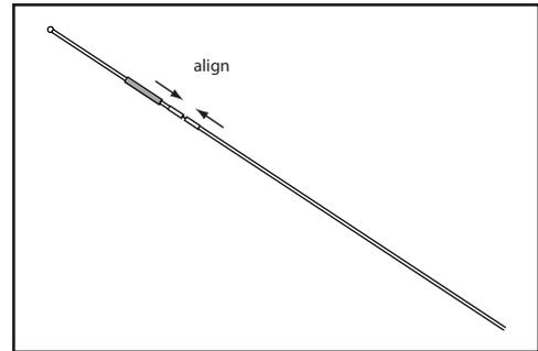
Figure 17-B: Aligning rod parts at the joint
