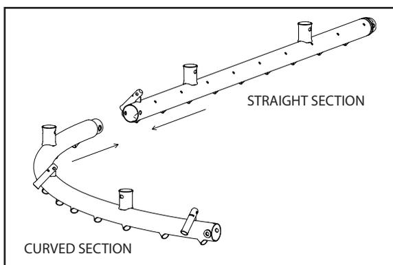
Figure 1: Joining curved section to straight section
