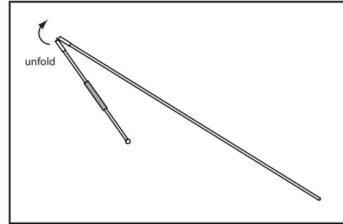
Figure 17-A: Straightening an enclosure rod
