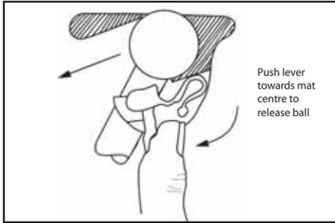
Figure 14-B: The release clip on the mat fitting
