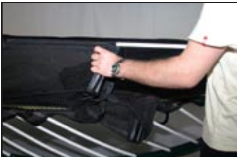
Figure 14: The horizontal rods being inserted into their sleeves in the enclosure
