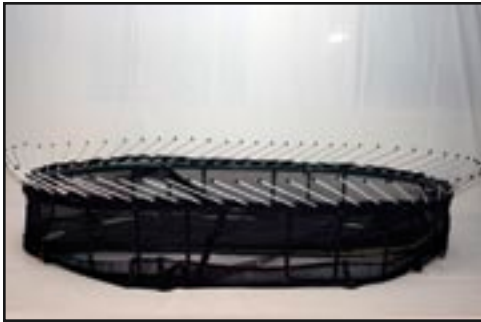
Figure 8: The rest of the rods inserted through the enclosure holes and into the frame sockets
