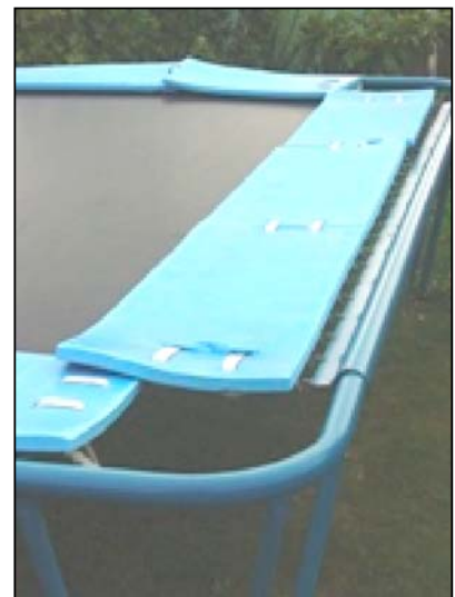
Figure 4: Unless anchored adequately, padding will move and will not prevent impacts with the frame.
