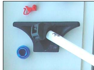
Figure 10: Plastic cleat ball-and-socket system for rod attachment to the mat edge. The clip (red) and the ball (blue) are shown separately.
