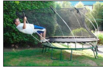
Figure 19: Tipping test of the SF40E with an over-the-weight-limit engineer climbing on the outside of the enclosure. Extra stability is provided by the splayed legs.
